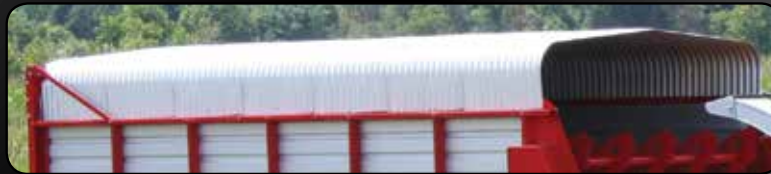
Formed roof molded with 20 ga Galvalume® for maximum rigidity
