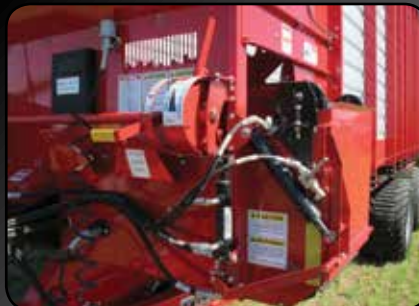
Hydraulic controls for cross conveyor extension, side conveyor and main apron
