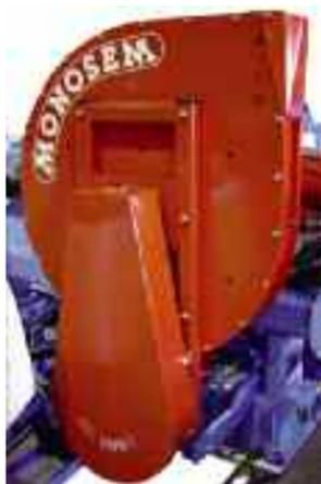
The extra high output turbofan offers the most volume of air. It is commonly used with planters that are 16-Row and larger. Can be used with either a PTO or a hydraulic motor. Most larger planters available with vacuum in the toolbar.
