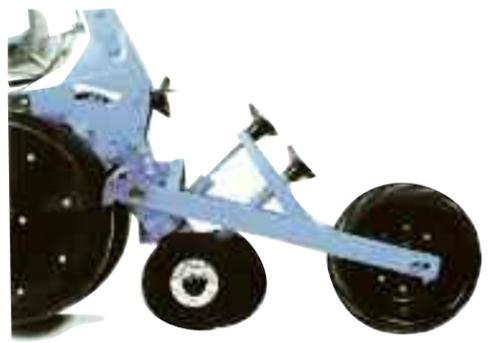
**V press wheel with disc closing system**
