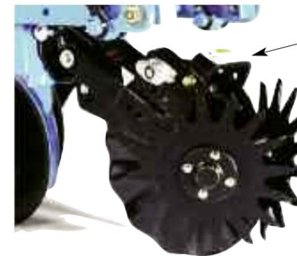
Quick adjust knob easily regulates depth control of the residue manager
