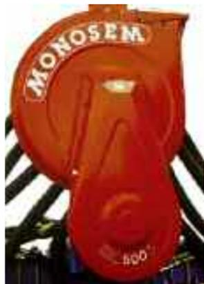
A high output turbofan with 12 or 16 outlets is available for larger machines that plant bigger seed or higher populations. Standard PTO speed of 540 rpm, on request 450 rpm and 1000 rpm. Optional hydraulic drive is available instead of PTO.
