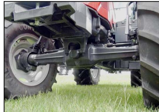
traction. Integrated front axle brakes are standard equipment to improve stopping power for safety.
